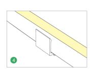
Fix led strip completely into the fixed clip,led strip subface must be parallel to the top edge of fixed clip.
